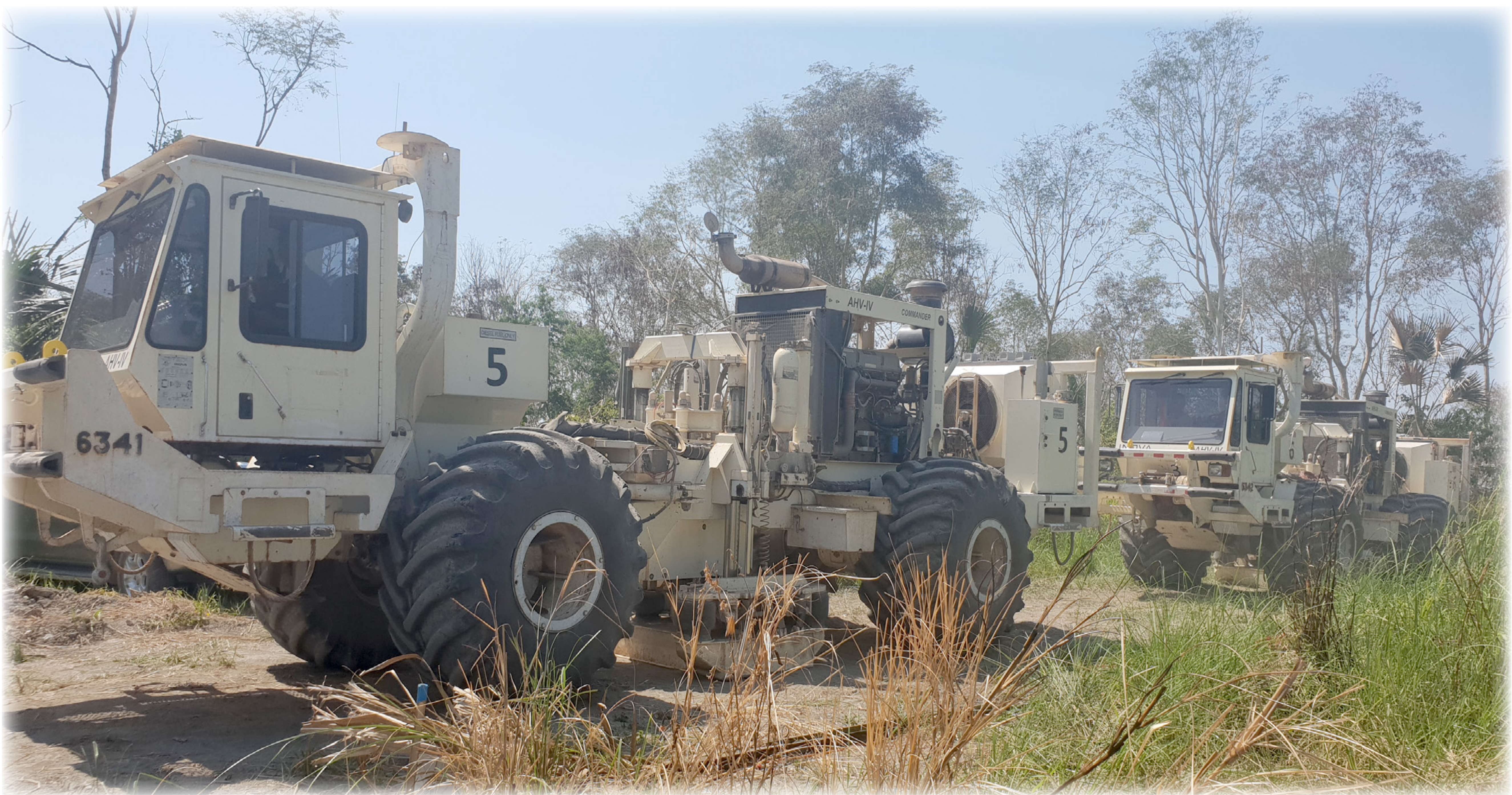
Figure 2-6: Vibroseis trucks during the 2D seismic acquisition in Block C
